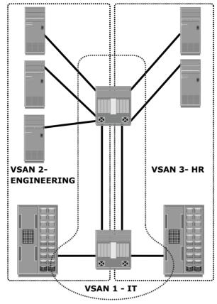
Figure 15-6: Securing SAN with VSAN
