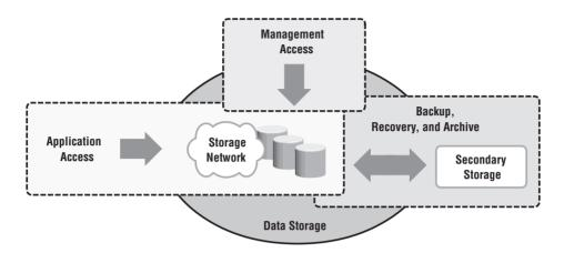
Figure 15-1: Three security domains of data storage
